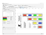
Packing patterns are defined simply by pulling the chosen product to the desired cavity on the blister pack. Up to four different products can be specified for a production order.
